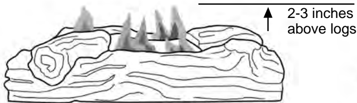
Fig. 22 - Correct Burner Flame Pattern
