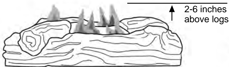
Fig. 31 - Correct/Normal Flame Pattern with short flames
